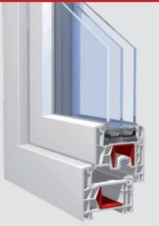
KBE 76 makes it easier and more convenient than ever before to achieve energy and heating cost savings. The new generation of windows can incorporate triple glazing and functional glazing up to a thickness of 48 mm. In other words: hardly any heating energy is lost through the glass. Yet the expansive glass surfaces allow valuable sunlight warmth to enter.
